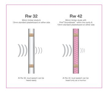
Rw is the weighted sound reduction in dB and it describes the airborne sound insulating power of a building element.
